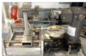
Fig.2 Apparatus for two-body sliding abrasion test
